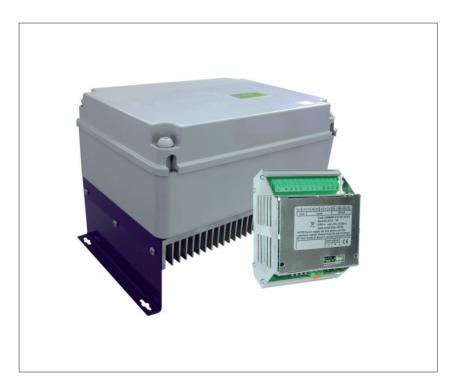
ACCSCS are designed to regulate the speed of fans and pumps proportionally and continuously. They function as a simple voltage regulator whose command signal (PWM for single phase controllers and 0..10 V or 4..20 mA or PWM for three phase controllers) comes from an external regulating device.
